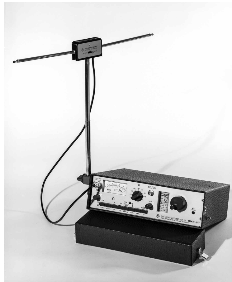
Fig. 6: HFV mobile VHF field strength meter with dipole antenna. This was not only the first fully solid-state Rohde & Schwarz measuring receiver, but also the first one able to perform automatic disturbance weighting according to VDE 0876.
