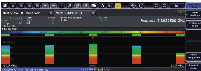
Fig. 3: Further measurement on the critical frequency using the multichannel APD measurement function. The 2D diagram provides a qualitative and quantitative result at a glance.
