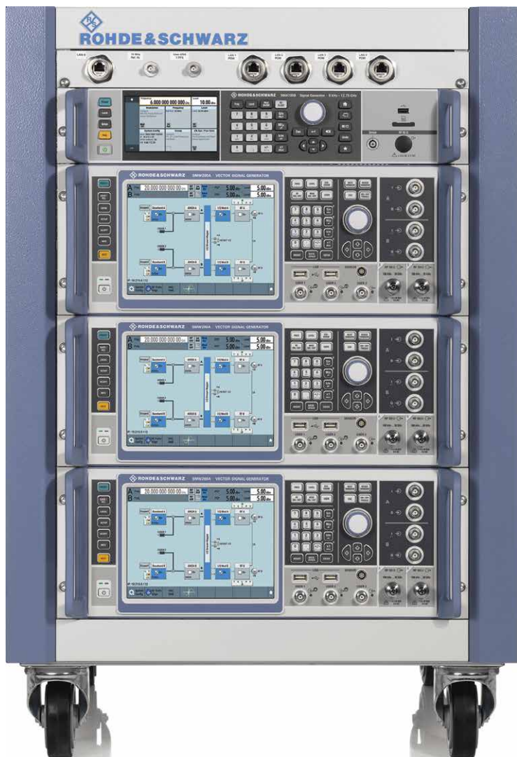
Fig. 3: A six-channel radar/GNSS test system consisting of three R&S®SMW200A vector signal generators and an R&S®SMA100B analog signal generator for the LO signal.
