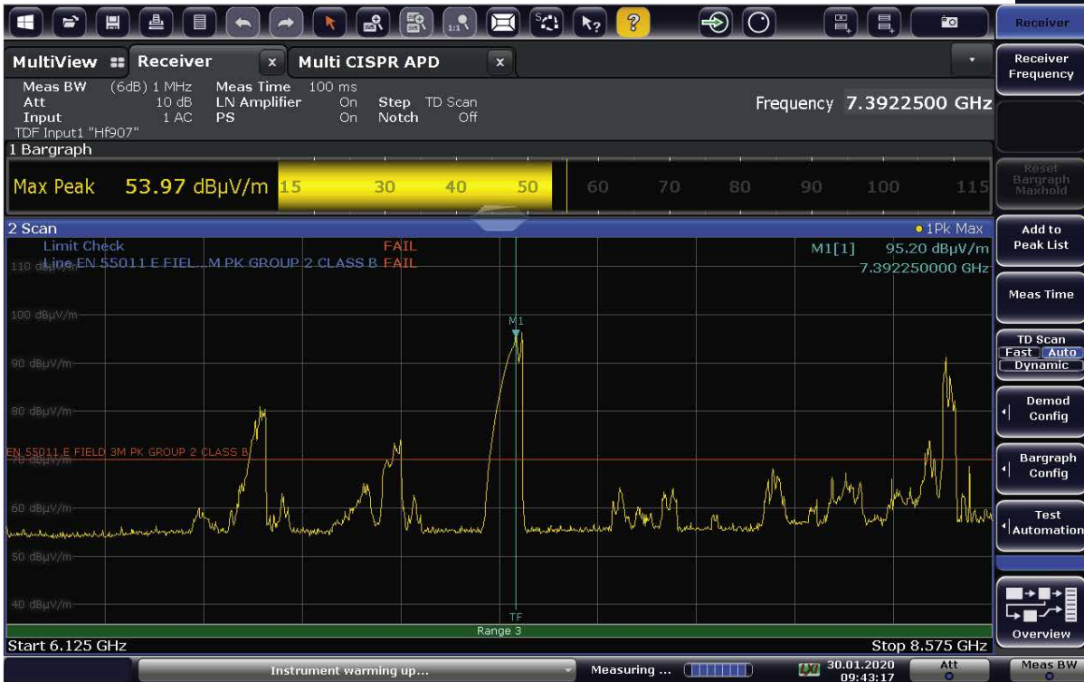
Fig. 2: Preview measurement on a micro-wave oven with the peak detector in subband 3 (6.125 GHz to 8.575 GHz). “FAIL” means that the measurement result exceeds the limit, so further APD measurement around the noncompliant frequency (here 7.39 GHz) is necessary.
